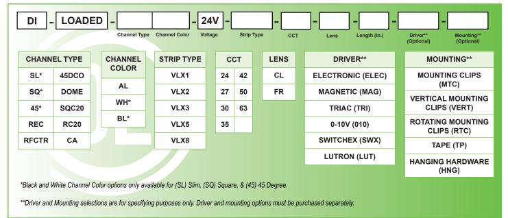
Example: DI-LOADED-SQBL-24V-VLX8-CL-36-SWX-RTC = Diode LED, Fully Loaded, Square, Black Channel, 24 Volt, VALENT<sup>®</sup> X 800, Clear Lens, 36 inches, 96" Lead Wire, SWITCHEX Dimmer, and Rotating Mounting Clips.
